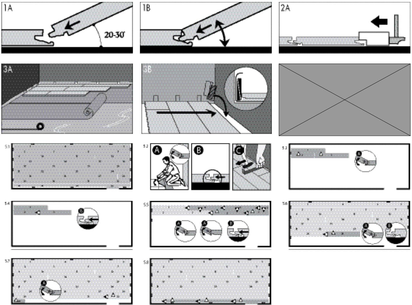
Work out the trims to be installed as some trims are easier to install prior to the flooring. This will be dependant on the direction of the trim to the flooring and the type of trim to be installed.
