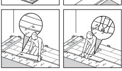
In places where it is too difficult to install the Uniclic® planks with the tapping block (e.g. against the wall), you can tap them together using the pulling iron and a hammer.
