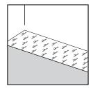
Underlay is essential for all laminate installations. The specially designed Quick-Step underlays have a damp-proof, insulating, noise-reducing and slight leveling function. The smooth top surface makes installing the laminate panels easier and allows the floors' expansion afterwards.
