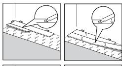
Continue now install the first board in the second row, ensuring that the end (or short) joins of any consecutive rows are at least 300mm apart to create a random staggered appearance and reduce wastage. Continue to install the boards as shown in the pictograms below and remembering to maintain the expansion gap using the spacers. After the first few rows are installed, use the offcut from the last row installed to start the next row.
