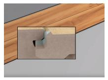
6. The locking system ensures a high, point and reliably prevents the join on the short profile springing out.
