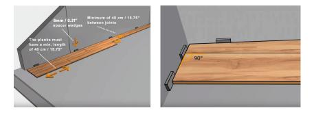
4. The first plank should be laid with tongue side adjacent to wall. The following planks should then be slid into place flat and horizontally.
