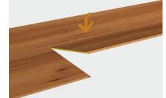
3. Always work the installation area from left to right. With this the tongue side should be beside the wall. Using spacer wedges ensure there is a constant expansion gap all round the floor of a minimum 8mm / 0.31"
